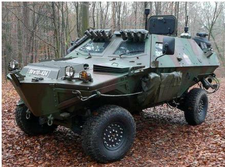
In Light Reconnaissance NBC Vehicle are integrated measuring instruments for NBC detection, system for sampling, system for contaminated field marking, radio and weapon station. The filtration system provides protection against NBC warfare agents for the crew (driver, operator and shooter). Light Reconnaissance NBC Vehicle is also amphibian armored vehicle.
