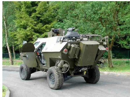
On the top of the armored vehicle automated weapon station is installed for inside crew protection and carrying out small missions.
